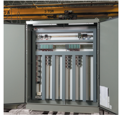
Remote I/O Enclosure
