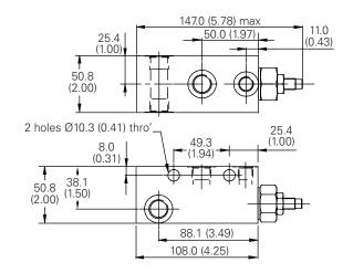
Note. Tightening torque of "F" adjuster locknut - 20 to 25 Nm Note. For applications above 210 please consult our technical department or use the steel body option.
