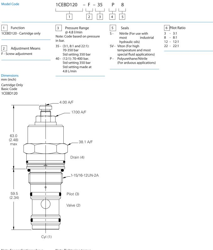
Note: For applications above 210 bar - please consult our technical department or use the steel body option Note: Tightening torque of "F" adjuster locknut -20 to 25 Nm
